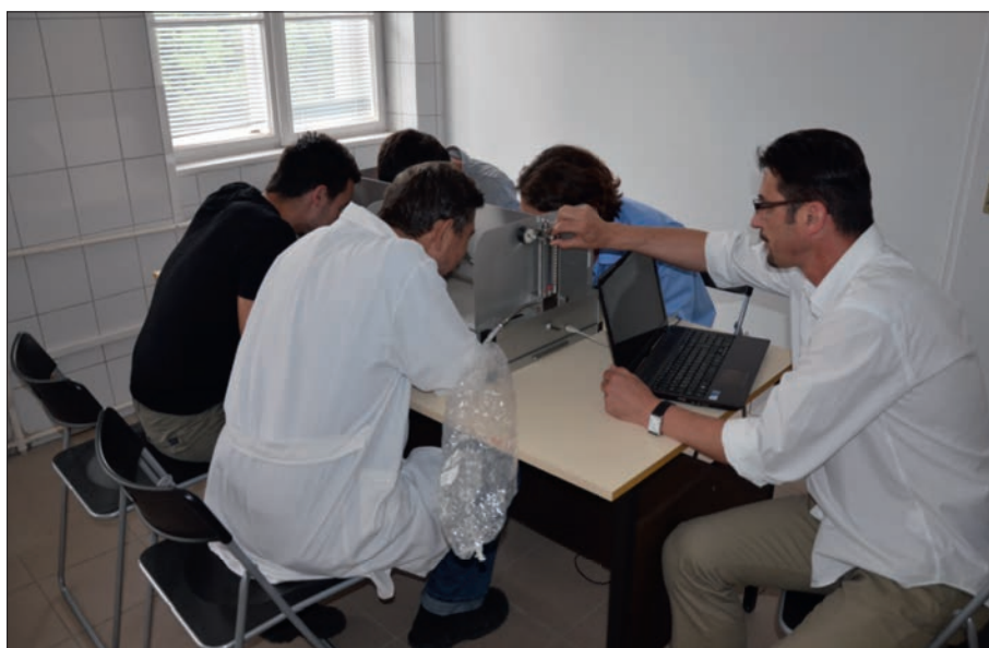
Figure 2. The dynamic olfactometer and persons involved in the measurement (Béres et al., 2014b)
